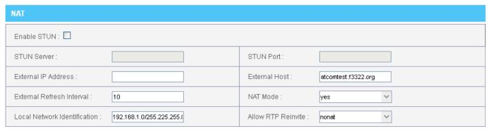
The External IP, External Host and Local Network Identification settings are used if you use IPPBX behind a NAT device to communicate with services on the outside.
